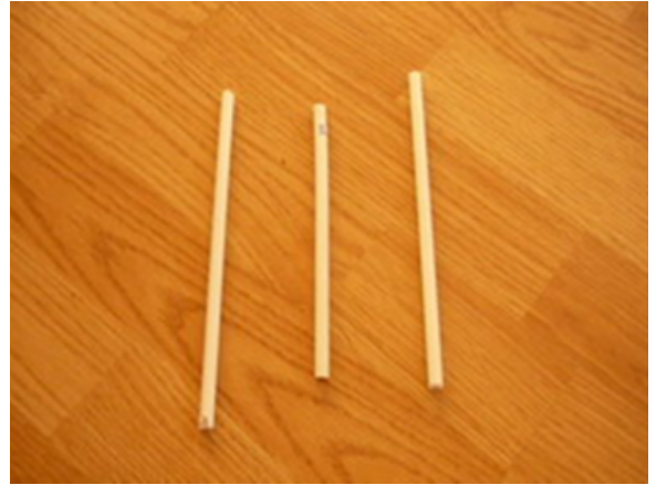
Fig. 2. Ceramic rods used for flame spraying.
