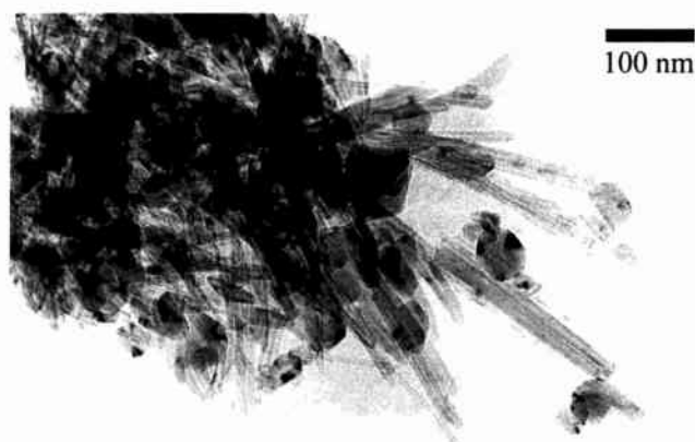
Fig. 1. TEM image of an agglomeration of MWCNTs and bucky onions from a sample grown using 40 A arc current.
